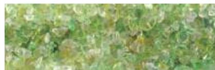
Using Glasspool,glass filter media, we get the most efficient filtration reducing the constant back washes and saving considerably the water consumption.
